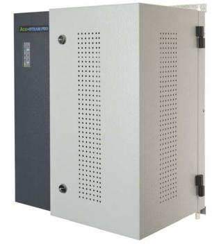
Acu-Steam Pro humidifiers produces humidity from steam dispersed directly into the air using electric elements immersed in water. By using resistive elements a wide range of water conditions can be used to generate sterile steam quickly and efficiently in a permanent stainless steel tank.
