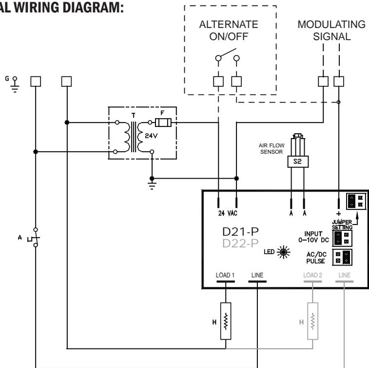
To switch the input between 0-10 VDC and AC/DC pulse, simply remove and replace the jumper according to the label. The D21-P has a single output with a maximum load as listed in the table below. The D22-P is equipped with two outputs effectively doubling the capacity of the D21-P. In cases with even larger loads, a D21-PS may be used instead to drive up to 4 SSRs. The maximum load is then limited to the capacity of the Solid State Relays.
