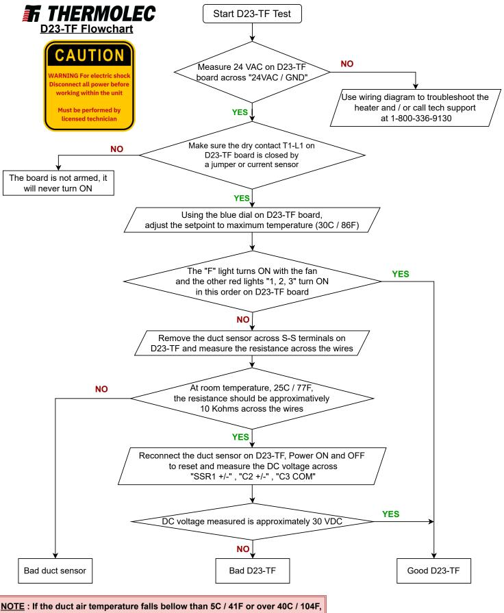
NOTE: If the duct air temperature falls bellow than 5C / 41F or over 40C / 104F the board D23-TF will turn OFF after one minute. The "W" light will start flashing once if the duct temperature is too low and twice if it is too high
